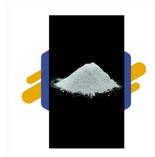
Quartz powder, derived from quartz crystals, exhibits exceptional properties that make it indispensable in diverse industrial applications. Its high purity, resistance to heat and chemical reactions, and electrical insulation properties render it ideal for use in electronics, ceramics, paints, and numerous other sectors. As such, the demand for premium-quality quartz powder continues to soar, driving the need for trustworthy manufacturers who can deliver consistent excellence.
